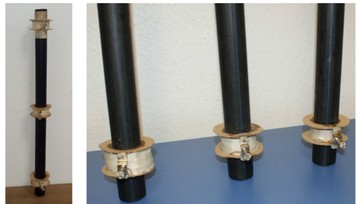
Figure 2: a) Set-up for experiment A: PVC tube with three identical coils attached to its top, middle and bottom. The coils have been assembled using cardboard. b) Set-up for experiment B: PVC tubes and attached coils with different number of turns.
