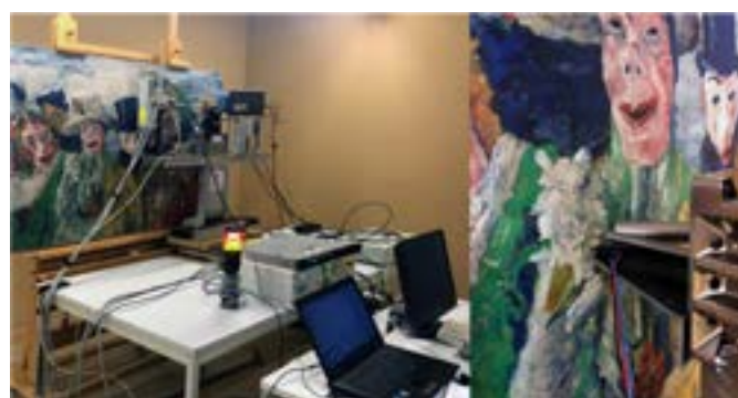
Left: Macro X-ray Powder Diffraction (MA-XRPD) scanner from the ARCHES and AXIS research group at the University of Antwerp, in front of The Intrigue (1890, KMSKA) by James Ensor. Right: Nozzle of the Macro X-ray Fluorescence (MA-XRF) scanner positioned close to the paint surface of the image.
