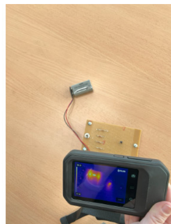
Set up of activity 1: using different equipment, the students identify the faulty resistor(s) in the circuit board.
