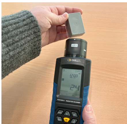
Set up of activity 4: examine radiation emitted by different objects. Image courtesy of the authors
