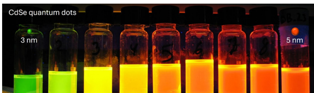
A series of vials containing CdSe quantum dots of increasing size ( \approx 3 -5 nm) in an organic solvent. Under UV light, their photoluminescence shifts from green to orange as their size increases.
