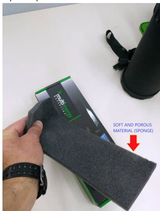
Figure 5: The reflective surface is completely covered by the sponge.
