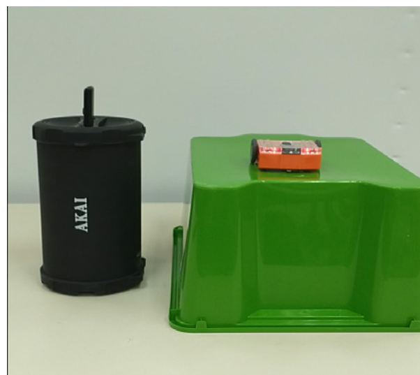
Figure 2: In the absence of the hard, smooth surface, the sound waves move upwards past the robot, which does not perceive the sound.
