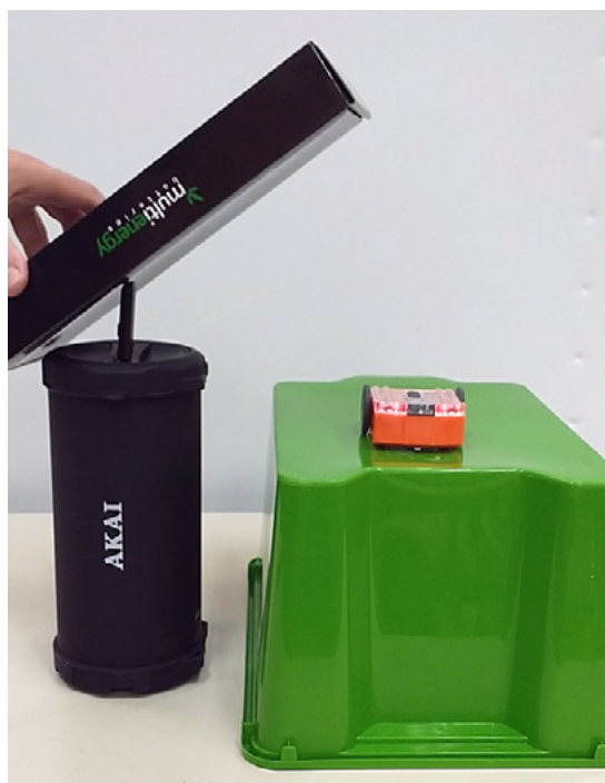
Figure 3: The smooth, hard surface is positioned to reflect the sound down to the robot.
