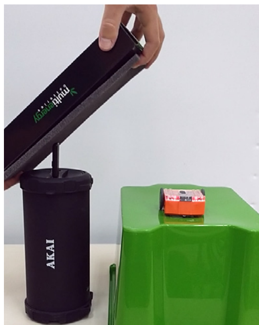
Figure 6: When the reflective surface is covered by the sponge, the sound waves don't reach the robot.
