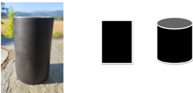
The projected area A_{\text{cp}} = \text{height} \times \text{diameter} of the cylindrical can = H \times 2r
