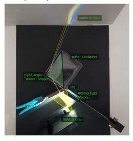
For this setup demonstrating light diffraction, it's not easy to identify all the elements from just the photograph, so the author has added some lines and notes to make things clearer.
