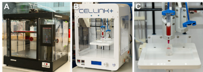
Some of the 3D printers used in our research cluster. A) A typical extrusion-based filament 3D printer. B-C) An extrusion-based 3D printer for biological applications, depicted while printing within an agarose gel support material.
