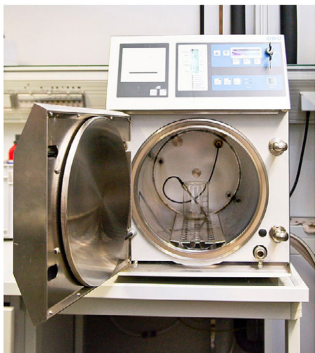
An autoclave for sterilizing laboratory or medical equipment. These large machines require a substantial amount of energy to manufacture and run.
