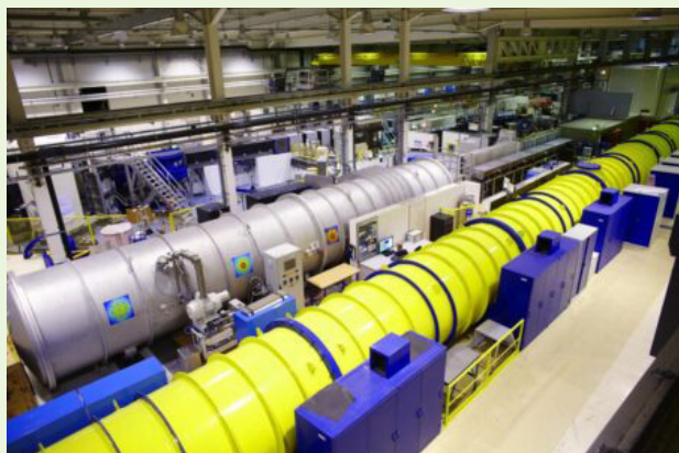
The SANS instrument D11 (long yellow tube) at ILL. © A Chezière/ILL
