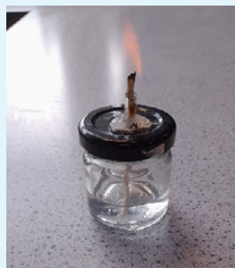
A homemade spirit burner Image courtesy of the author
