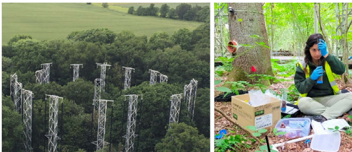
Figure 3: Left: The Birmingham Institute of Forest Research-FACE (BIFoR-FACE) facility in the UK. Right: A researcher on site, labelling soil with a nitrogen isotope ( ^{15}\text{N} ) to measure nitrogen fluxes.
