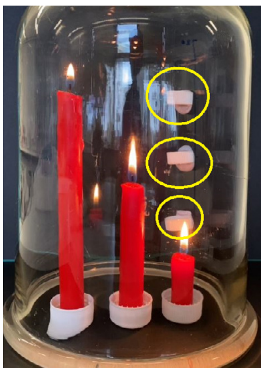
Figure 5: Monitoring the CO 2 concentration in the gas jar Image courtesy of the author
