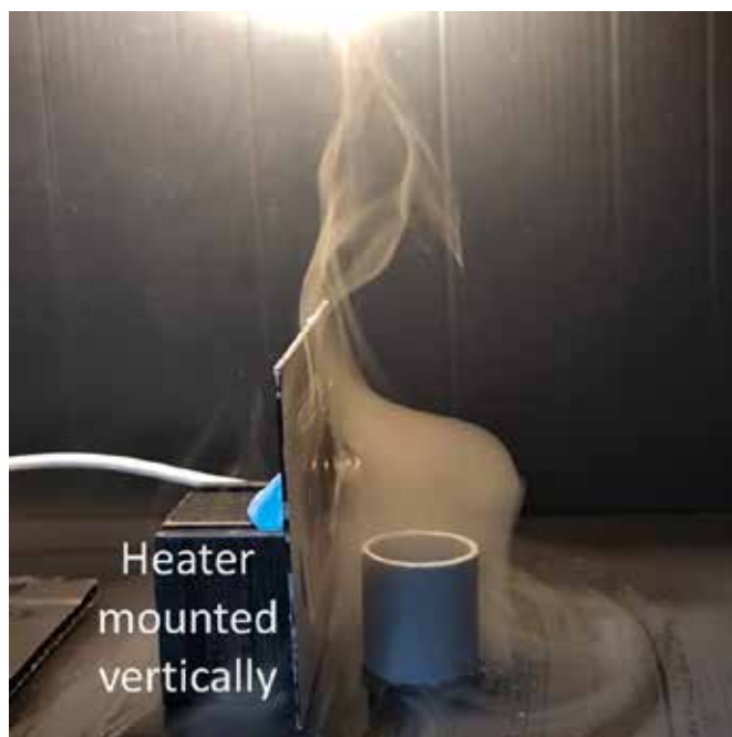
Figure 3: Testing the explanation that mist is pushed away by radiation. As the heater is positioned vertically, most radiation from the heater moves horizontally to the right. Since the mist does not move preferentially to the right, the explanation is false. Additionally, we observe that the mist rises near the heater, supporting the original explanation of warm air rising, bringing the mist along with it.
