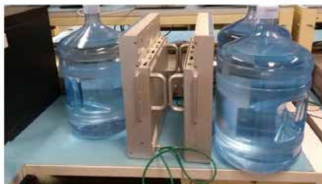
Left: The portable neutron detectors for the aircraft, consisting of two blocks of 12 cylindrical proportional counters.
