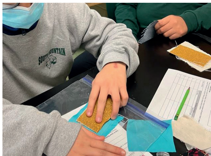
Students checking the durability of the fabric material. Here, sand paper is applied to the fabric, but wrapping the fabric around a ball and rubbing it against the sandpaper works better. Image courtesy of Ivonne Miranda
