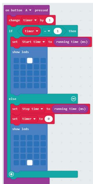
Figure 5: Recording the start and stop times in variables
