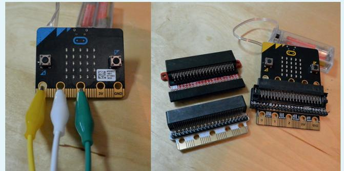
Figure 2: Alligator clips (left) to add devices and expansion boards (right) to add devices/components
