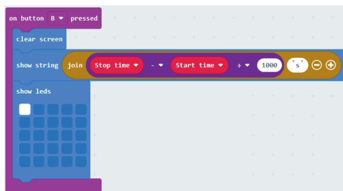
Figure 6: Calculating and showing the elapsed time
