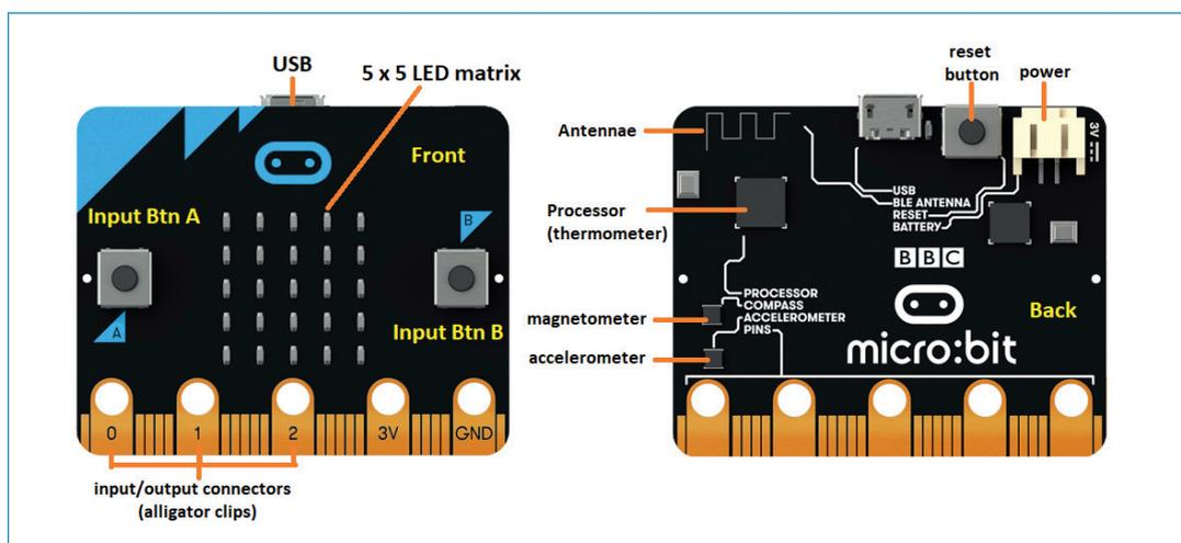
Figure 1: Front and back of micro:bit (version 1)
