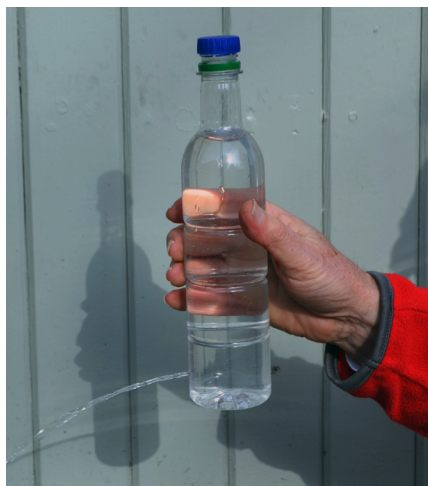
Figure 4: Holding the bottle with a hole at the base: a jet of water flows out.
