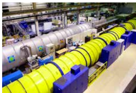
The SANS instrument D11 at ILL, which was used for the limoncello study
