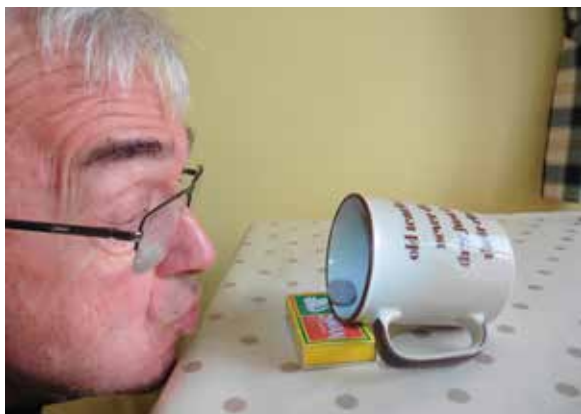
Figure 2: The coin is lifted into the cup by the reduction in air pressure above it.
