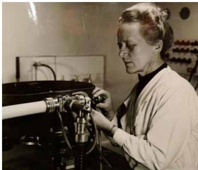
Ida Noddack-Tacke adjusting an X-ray spectrometer in the laboratory, 1944
