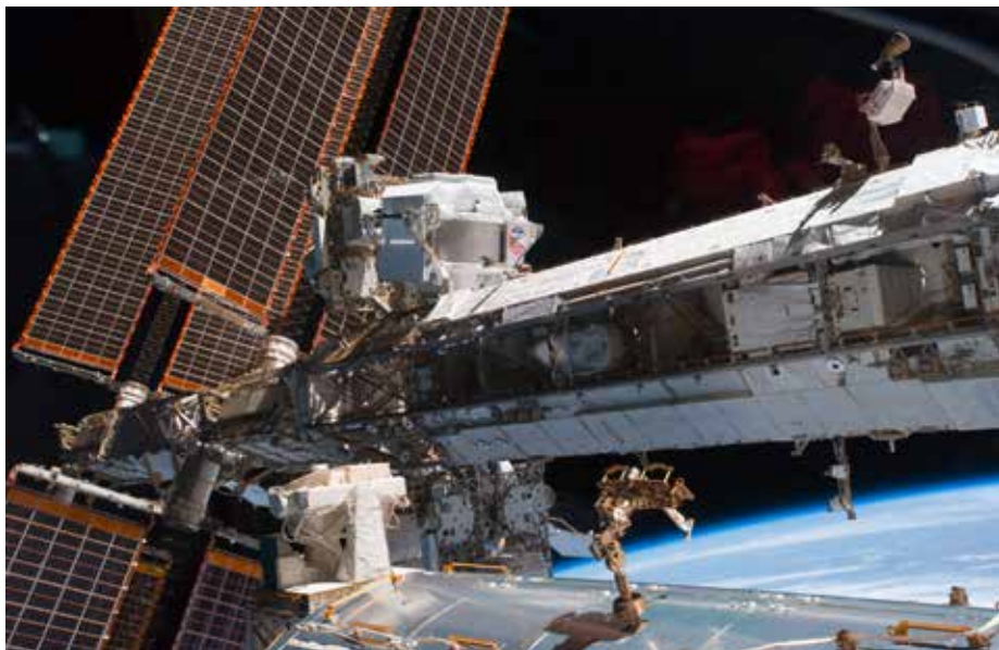
The Alpha Magnetic Spectrometer (centre left) on the International Space Station.
