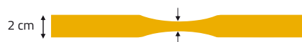
Figure 1: Two pieces of aluminium tape are cut to the length of the salad bowl and so they are narrower in the centre.
