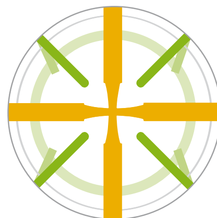
Figure 4: Connect the narrow strips of aluminium tape on the outside of the bowl using the four remaining strips.
