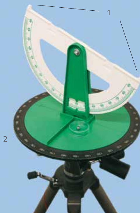
Figure 1: a theodolite, with sights (1) and turntable (2)
