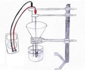
8. Set the voltmeter to  $\pm 200$  mV and observe.
