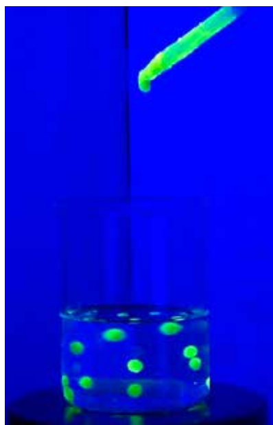
Figure 4: Luminescent bubbles under UV light
