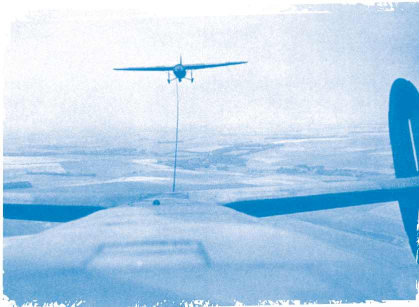
Gliders need to be towed in the air, usually by being attached behind a plane, before they can fly on their own. This photo of a glider was taken from the towing plane and shows the rope linking them.
