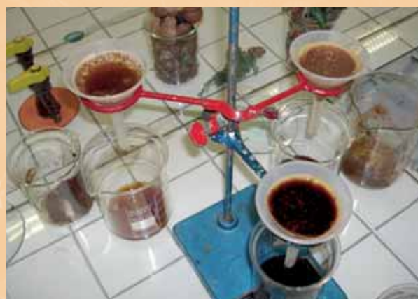
Figure 5: Filtering the water and crushed gall mixture
