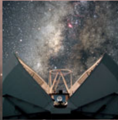
The Faulkes Telescopes each weigh 25 tonnes, stand 8 metres tall with 2 metre primary mirrors, and are contained within a novel clamshell enclosure
