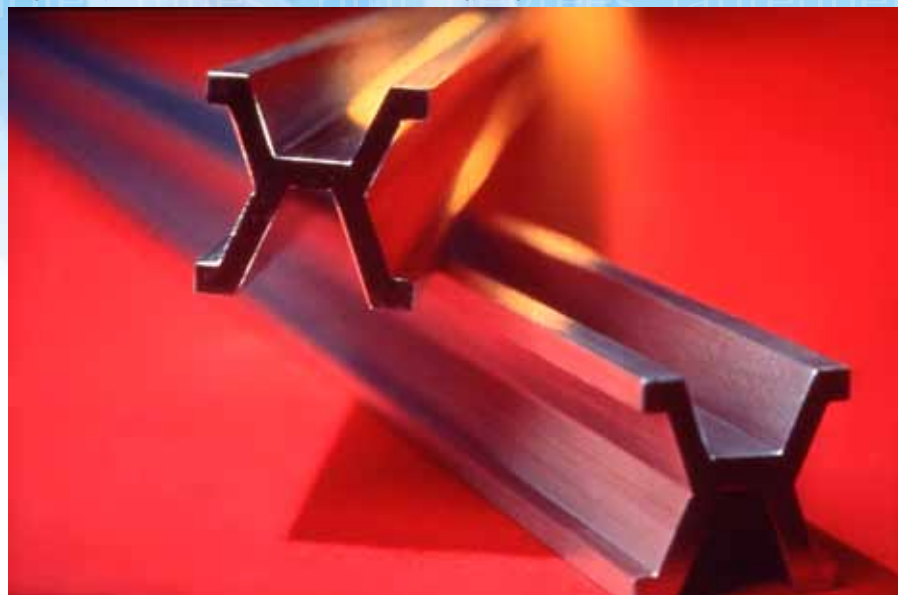
Figure 1: The international prototype metre bar, made of an alloy of platinum and iridium. This bar embodied the international definition of a metre from 1889 to 1960.
