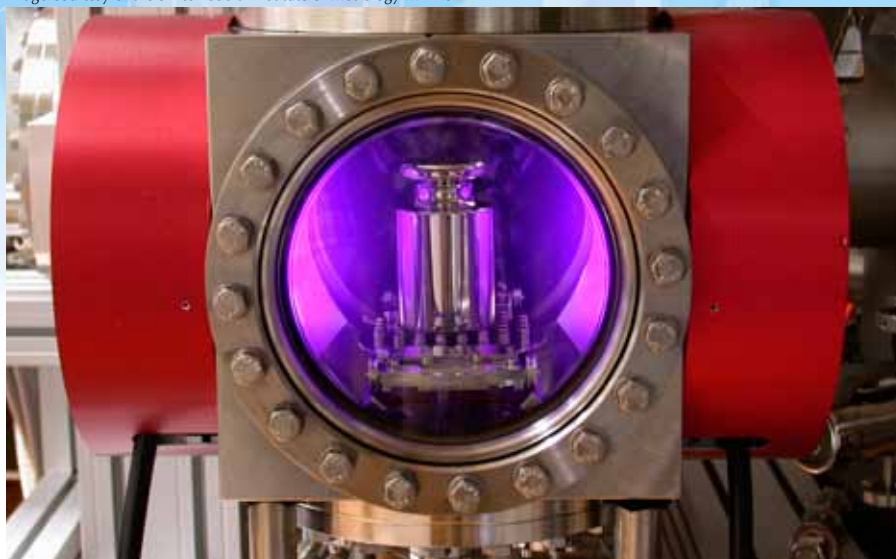
A mass prototype is getting a thorough clean in low pressure plasma.
