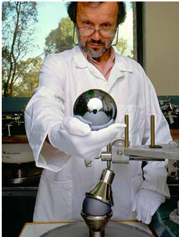
Figure 4: One of the scientists at the Australian Centre for Precision Optics holding a 1 kg silicon sphere for the Avogadro project, an international collaboration to define the kilogram. This sphere is one of the roundest man-made objects in the world.
