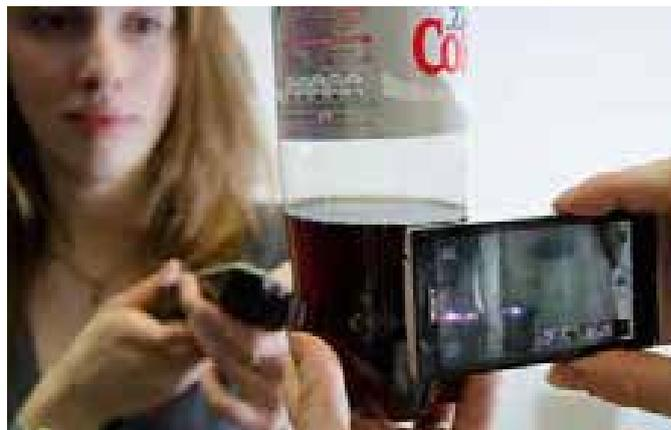
Although visible light from a torch is absorbed by cola, infrared radiation is not
