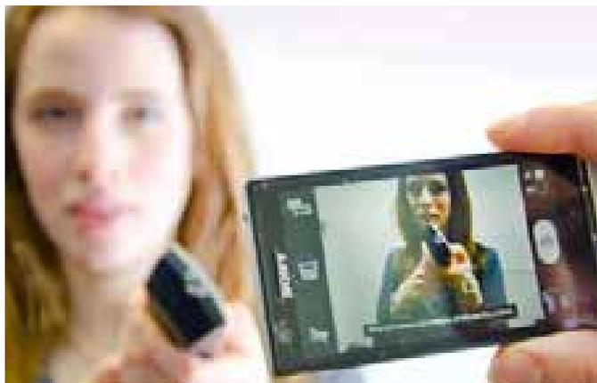
Unlike your eyes, a digital camera will register the infrared radiation from a TV remote control
