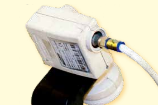
Figure 8: Powering the satellite meter and receiving the signal from the LNB
