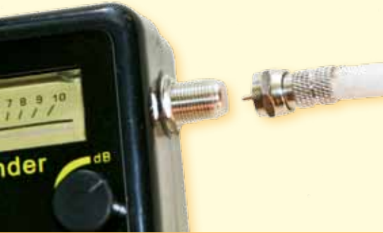
Figure 6: Attaching the LNB to the satellite signal meter
