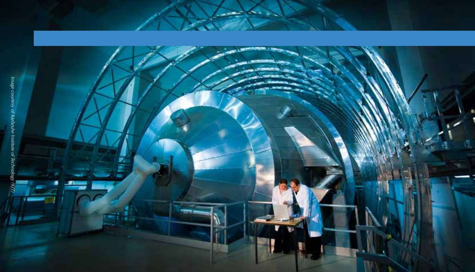
The KATRIN spectrometer in Karlsruhe, Germany, is one of the experiments aims to 'weigh' neutrinos
