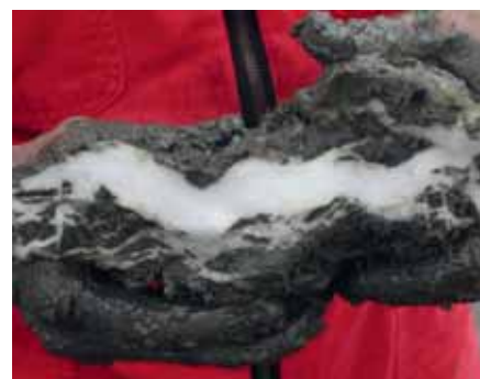
White gas hydrates consolidate sea floor sediments
