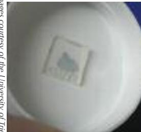
Figure 3: CR39 inside the ‘exposure camera’
