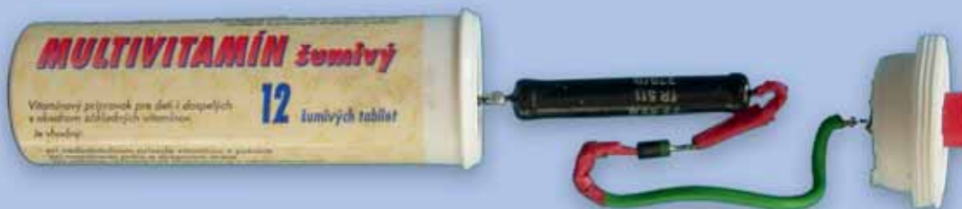
Figure 2. Construction of the black box
