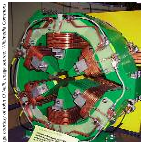
Sextupole magnets are used for correcting the beam size and position
