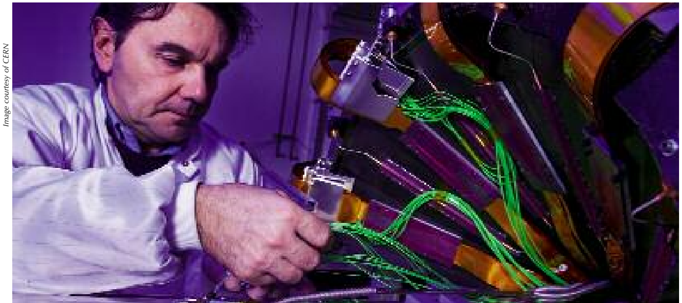
Integration of the ALICE experiment's inner tracker
