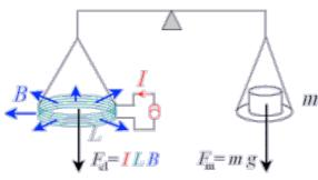
The static weighing phase Image courtesy of the BIPM
