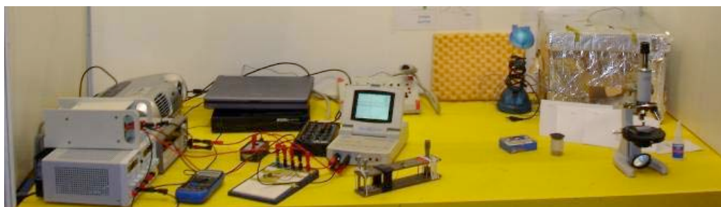
The full setup (from left to right): two power supplies, the signal generator with a projector for demonstrations (optional) on top, the NI DAQcard (in black) with the computer on top, the current card (the two small black boxes and one black and white box in the centre), the oscilloscope (with the screen) and the microscope stand. The small blue box is an optional instrument used to check the current. It is not part of the actual circuit / setup. On the right-hand side, you can see the microscope and glue we use for preparing the tungsten tips and an aluminium foil-covered cardboard box with insulating expanded polystyrene inside, which we used to isolate the microscope stand from vibrations and the electromagnetic field. Because we did not notice better performance when using the box and we realised that the current used is in fact strong enough and is not disturbed easily by further electromagnetic fields, we stopped using the box
