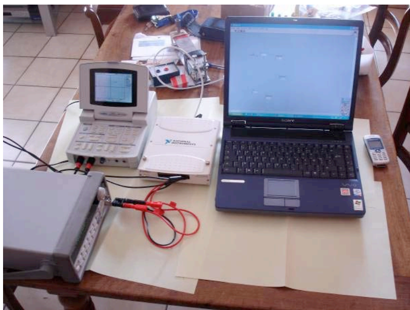
Our first setup (from left to right): the signal generator, the oscilloscope, the National Instruments (NI) DAQcard and the computer. In the background, you can see the actual microscope stand. To use the microscope, it needs to be placed on the floor – on top of a table, the vibrations are too strong
