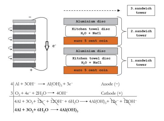
The voltaic pile and the half equations for each electrode, along with the overall balanced reaction Image courtesy of the author
